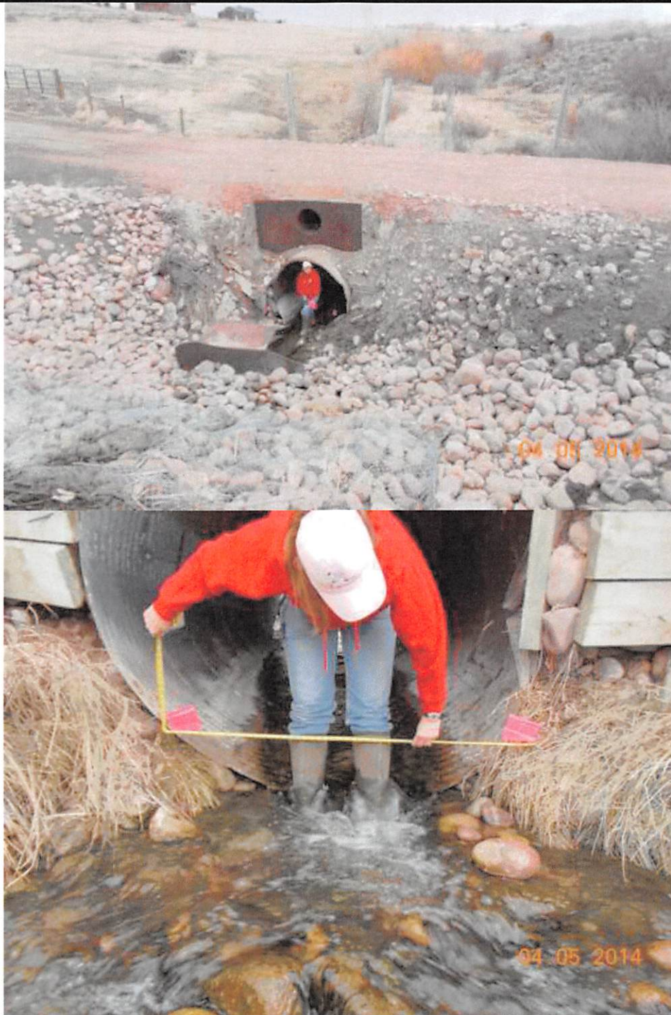
Top Photo: East facing view of Dr. Kagel standing in outflow channel below dam. Bottom Photo: Close-up western view of Dr. Kagel measuring OHWM width.
