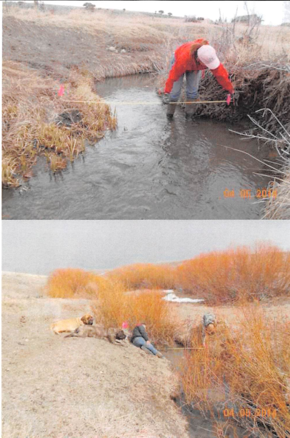
Top Photo: East view of downstream channel width (84") at the OHWM. Bottom Photo: Downstream (east) view of the channel above the pond.
